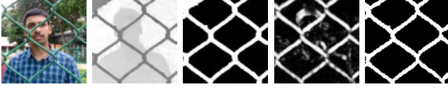
Fig. 9. (a), (b) RGB image and its corresponding depth profile obtained from the light field data captured using Lytro. (c) Binary segmentation mask obtained from (b) using Eq. (3). (d) Segmentation mask generated by feeding (a) to the proposed end-to-end CNN. (e) Final binary occlusion mask obtained by combining both (c) and (d), respectively.
