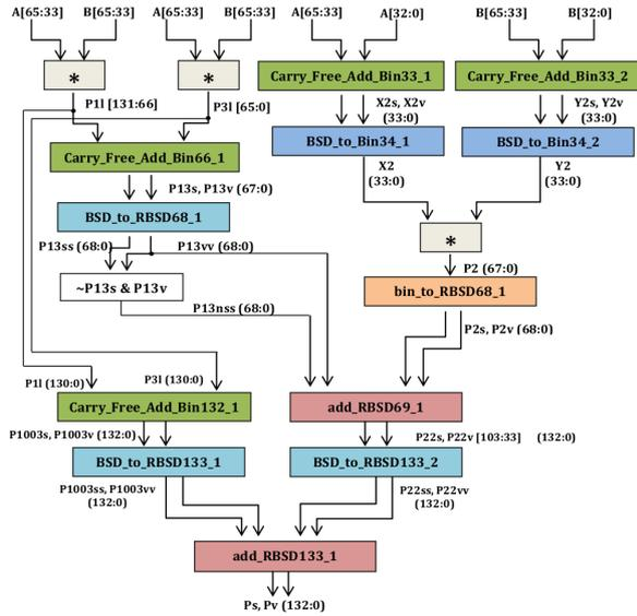
Fig. 1. Circuit design of carry-free multiplication of binary numbers.
